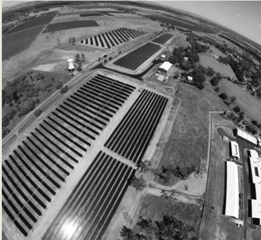
UQ's 3.275 megawatt solar photovoltaic systems research facility, located at Gatton campus. Image: Adam Harper.
